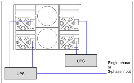
Figure 73: Single basic unit with two UPSs
